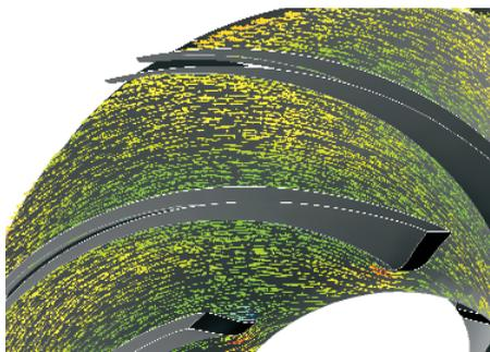
Relative velocity vectors on a plane between the rotor blades
