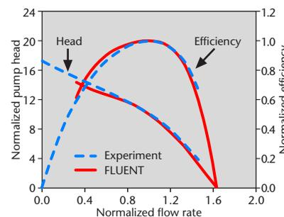
Comparison of pump performance and efficiency with data
