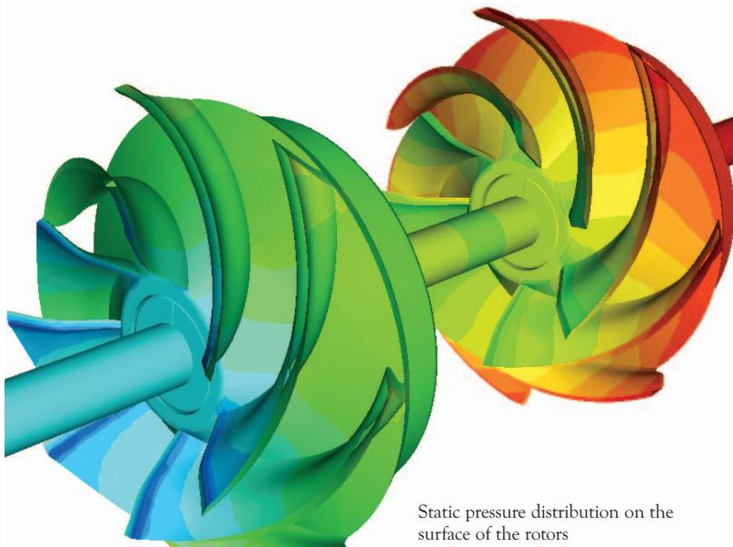
Static pressure distribution on the surface of the rotors
