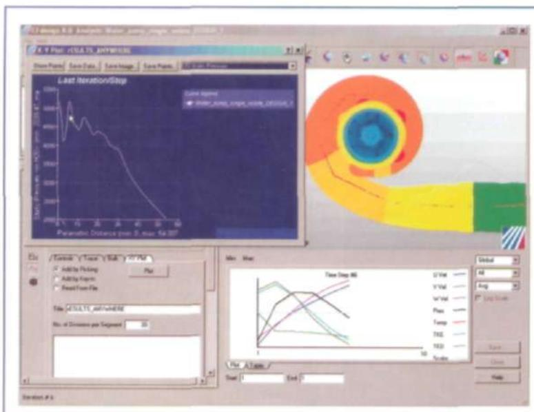
Figure 2. Virtual probe plotting anywhere inside the machine to show any result.
