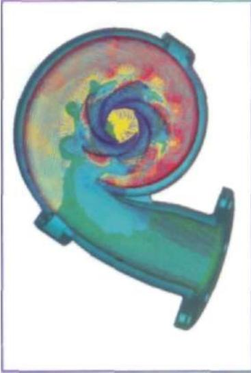
Figure 4. Cross-section view showing flow vectors and excessive separation at cutwater.
